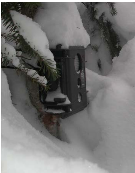
Figure 4. Reconyx remote camera with infra-red detector and flash.
